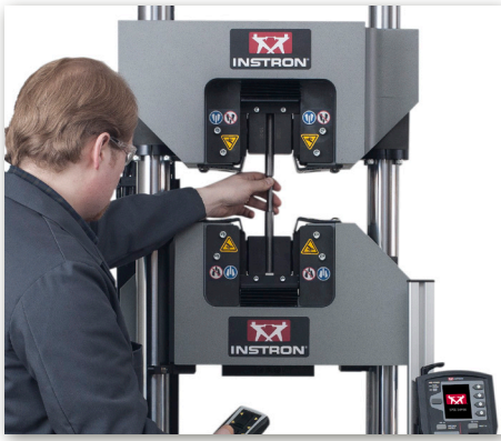
G7 - Open Front with Hydraulic Actuation
